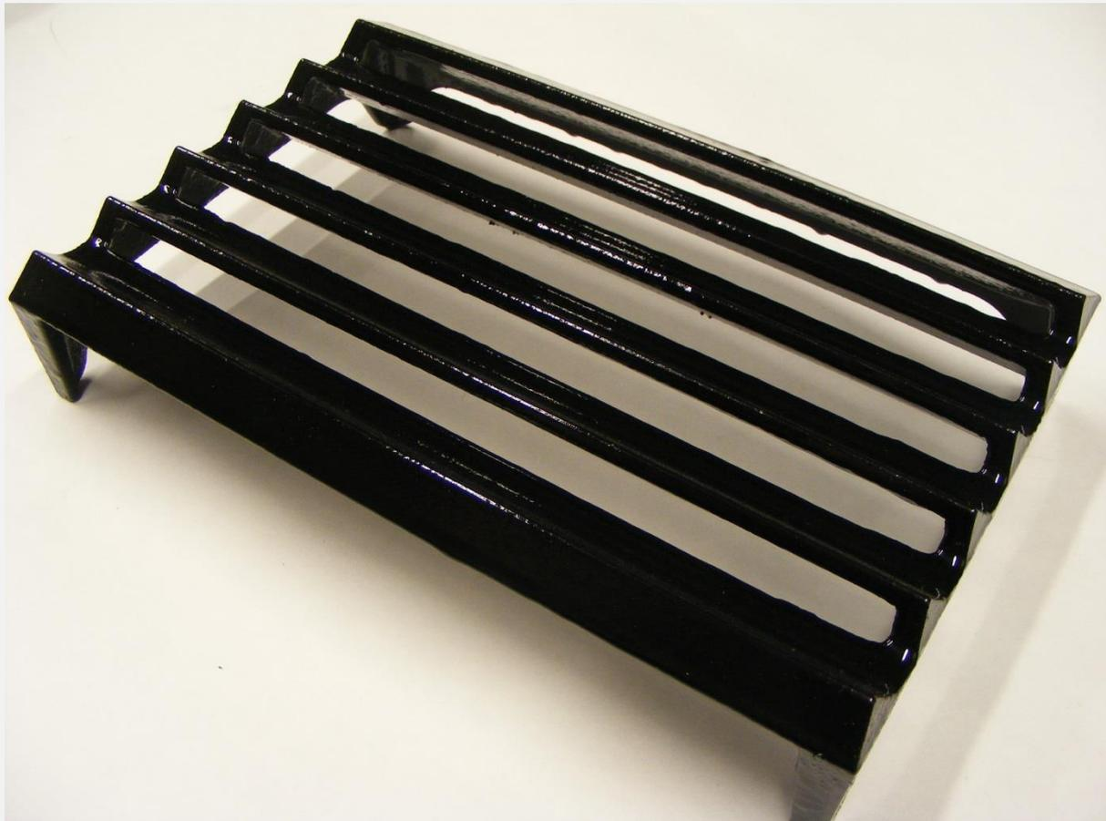
Cast iron louvre air bricks are made from grey iron, cast in sand moulds bonded with resin to a fine cast finish and are available in three sizes (9x3, 9x6 and 9x9) (see table below for metric mm sizes).
