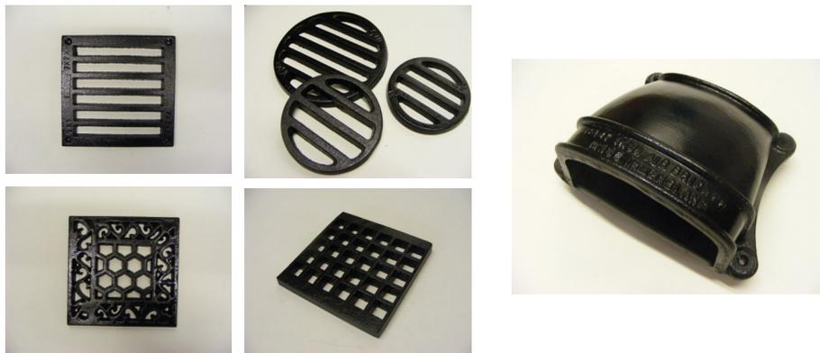
Our cast iron grilles are flat plates and once drilled are perfect to conceal core drill holes for extractor vents of 4" (100mm), 5" (125mm) and 6" (150mm) diameter. The core drills required for the corresponding vent pipes will need to be slightly larger than the pipe at 107mm, 127mm and 152mm diameter respectively.
