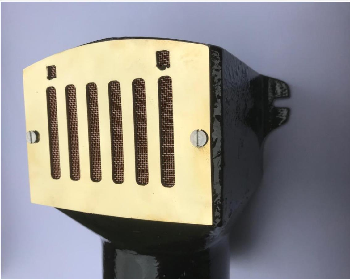
Cast iron cellar and soil vents are made from grey iron, cast in sand moulds bonded with resin to a fine cast finish and are available in one size with different options for the front plate.
