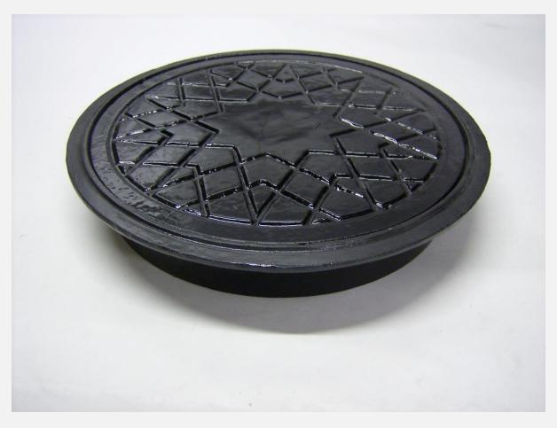
Cast iron coal hole covers and frames are made from grey iron, cast in sand moulds bonded with resin to a fine cast finish and are available either solid or vented with or without the frame.
