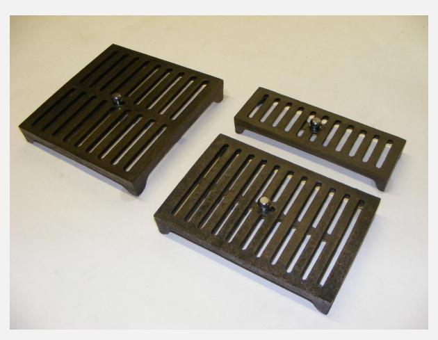
Cast iron hit and miss air bricks are made from grey iron, cast in sand moulds bonded with resin to a fine cast finish and are available in three sizes (9x3, 9x6 and 9x9) (see table below for metric mm sizes). This is the only cast iron air brick available which has a movable shutter.
