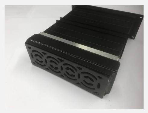
Used with the periscope duct (item PER) it is essential to use the METIMP adapter as the back of the REG3 air brick has cut away shoulders and wouldn't sit flat on the sleeve, duct tape is also essential as the fit of the air brick in the adapter is loose and the adapter is loose fitting on the periscope duct.
