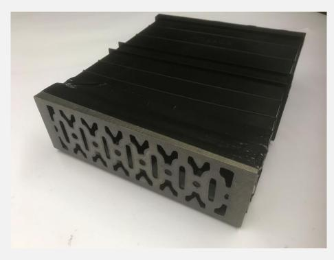
Used with the periscope duct (item PER) it is essential to use the METIMP adapter as the back of the Y3 air brick has cut away shoulders and wouldn't sit flat on the sleeve, duct tape is also essential as the fit of the air brick in the adapter is loose and the adapter is loose fitting on the periscope duct.
