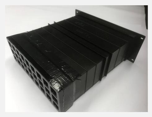
Used with the periscope duct (item PER) the METIMP adapter is not required. The back of the MAX3 air brick has a flat box that sits against the sleeve and can be duct taped into position. The periscope duct reduces the free area of the MAX3 by 50mm2 to 7750mm2.
