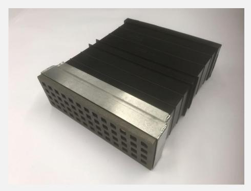
Used with the periscope duct (item PER) it is essential to use the METIMP adapter as the back of the GRID3 air brick has cut away shoulders and wouldn't sit flat on the sleeve, duct tape is also essential, the fit of the air brick in the adapter is very good but the adapter is loose fitting on the periscope duct.
