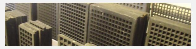
Cast iron long gratings and grilles are made from grey iron, cast in sand moulds bonded with resin to a fine cast finish and are available in various widths. They are imperial so are predominantly available in 3ft lengths. They are used either laid vertically for ventilation or laid flat as drainage gratings for walkways and pavements.
