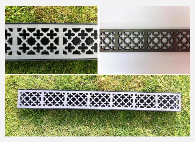
Cast iron channel grating grilles are made from grey iron, cast in sand moulds bonded with resin to a fine cast finish and are available in various lengths up to a maximum of a metre and can be used with or without the plastic channel.
