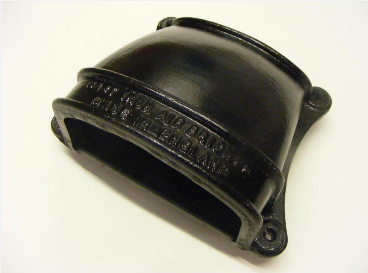
Cast iron conservation vents are made from grey iron, cast in sand moulds bonded with resin to a fine cast finish and are available in one size with two different diameter spigots at the back 100mm dia (4" item CON4) and 125mm dia (5" CON5).
