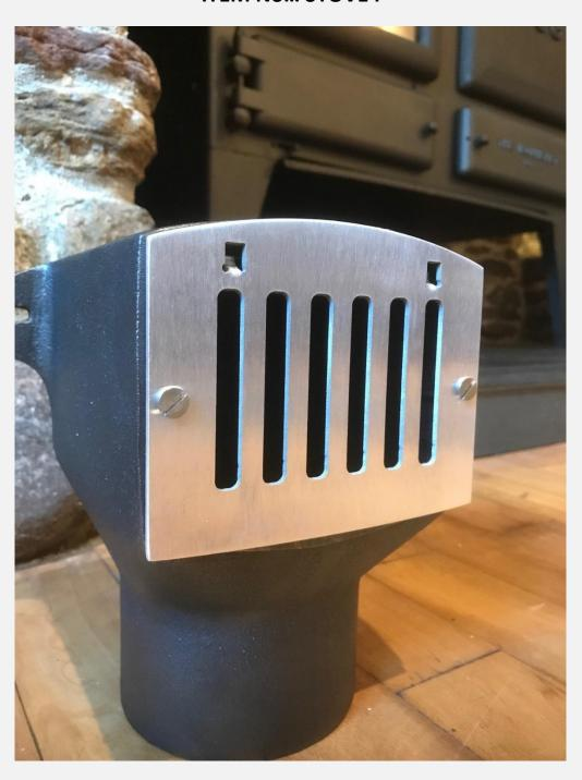
Cast iron stove and log burner vents are made from grey iron, cast in sand moulds bonded with resin to a fine cast finish and are available in one size with different options for the front plate.
