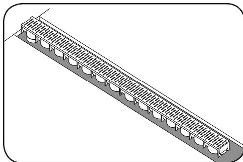
**2.** Align the chosen exit point with the drain outlet and slot into place, bedding the channel down into the concrete base. Lay the adjacent channels, bedding down as you go. Joints between channels should be sealed with a suitable silicon or polysulphide sealant. Once bedded, haunch the channels in place to fully support the side walls of the channel.
