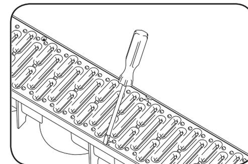
**8.** To remove the grate, use a flat blade screwdriver at the clip points to ease the clips open. The grate can be further secured using 4 3.5 x 30mm self tapping screws.
