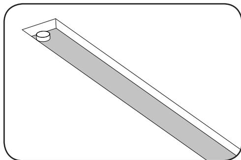
**1.** With an appropriate silt trap installed, dig a trench to the sizes detailed in Fig. A for the required run length. Pour a layer of semi-dry concrete in the bottom of the trench to the depth shown, the concrete used should be to the strength of a C25 mix. The top of the channel should lay 3-5mm below the top level of the paving material once installed.
