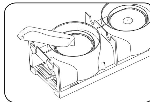
**3.** To remove the appropriate exit point, use either a heavy duty knife or 80mm hole saw prior to installing the channel.
